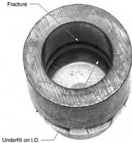
Fig. 40 Photograph of a back extruded part. Note the severe circumferential fracture (dark area) and die underfill (below dark area) on the inside diameter (ID).
