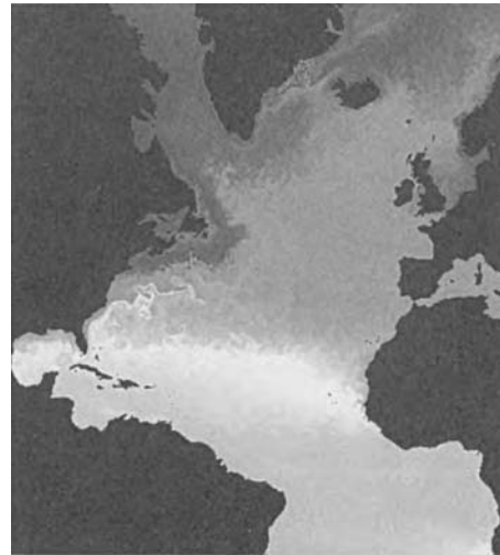
Fig. 2 Ocean surface temperatures from a recent computational fluid dynamics simulation of the North Atlantic Ocean. Source: Ref 8
