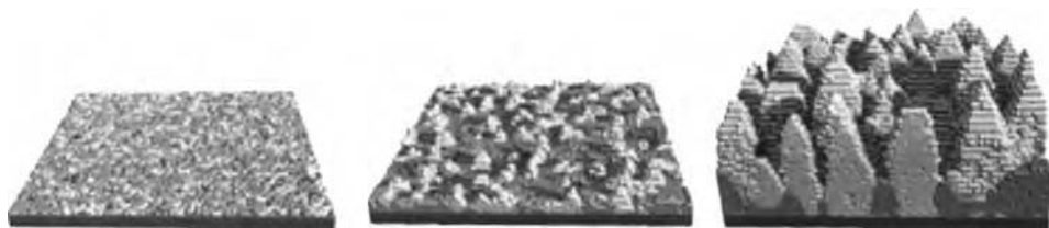
Fig. 17 Growth of aluminum onto a flat substrate (dark gray) with a cosine angular distribution for the impinging aluminum atoms. (001) clusters (light gray) and (111) clusters (intermediate gray) are permitted to nucleate and grow simultaneously using a multilattice model. Configurations from left to right correspond to film at various times. Source: Ref 159
