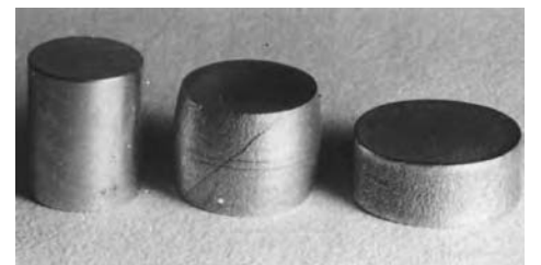
Fig. 15 Compression tests on 2024-T35 aluminum alloy. Left to right: Undeformed specimen, compression with friction (cracked), compression without friction (no cracks)
