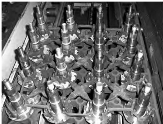
Fig. 27 Comparison of existing and proposed racking of automotive pinions
