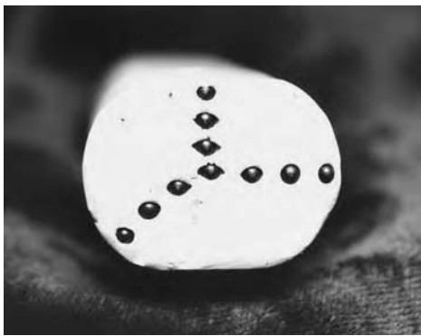
Fig. 38 Plasticine ingot representing side pressing of a K-Monel ingot. Hard beads have been embedded to illustrate the presence of tensile stresses at the center of the ingot. Damage seen is directly related to the tensile stresses.
